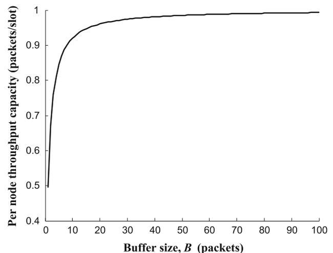
**Fig. 5** Illustration of per node throughput capacity varying with buffer size in a large-scale ad hoc network
