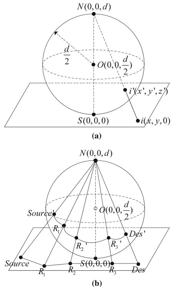
**Fig. 7** Illustration of the LCSR routing scheme. **a** Reversed stereographic projection. **b** Routing selection
