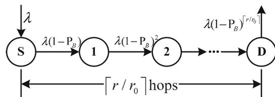
**Fig. 4** Illustration of the impact of self-generated packets on the whole network
