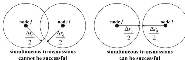
Fig. 3 Illustration of the essential condition of simultaneous successful transmissions
