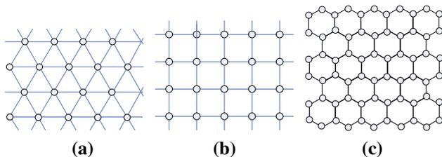
**Fig. 6** Illustration of symmetrical network topologies. **a** Regular triangle. **b** Square. **c** Cellular
