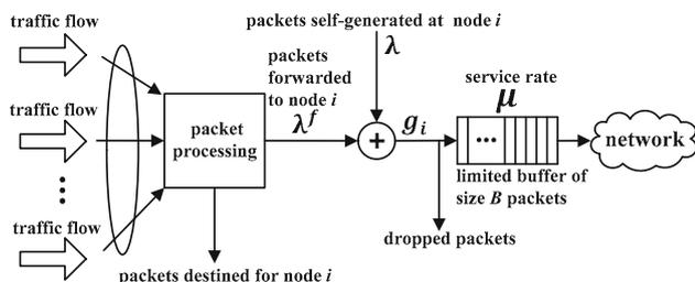
Fig. 2 Illustration of the  $G/G/1/B$  queuing model
