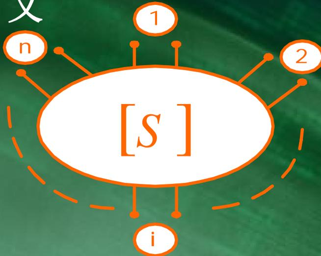
$$\begin{bmatrix} b_1 \\ b_2 \\ \mathbf{M} \\ b_n \end{bmatrix} = \begin{bmatrix} S_{11} & S_{12} & \mathbf{L} & S_{1n} \\ S_{21} & S_{22} & \mathbf{L} & S_{2n} \\ \mathbf{M} & \mathbf{M} & \mathbf{M} & \mathbf{M} \\ S_{n1} & S_{n2} & \mathbf{L} & S_{nn} \end{bmatrix} \begin{bmatrix} a_1 \\ a_2 \\ \mathbf{M} \\ a_n \end{bmatrix}$$
