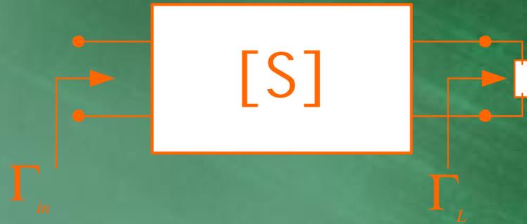
$$\Gamma_{in} = S_{11} + \frac{S_{12}S_{21}\Gamma_L}{1 - S_{22}\Gamma_L}$$
