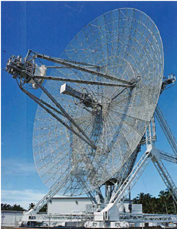
Figure 4. A long-range radar antenna, used to track space objects and ballistic missiles. (Source: Wikimedia Commons.)
