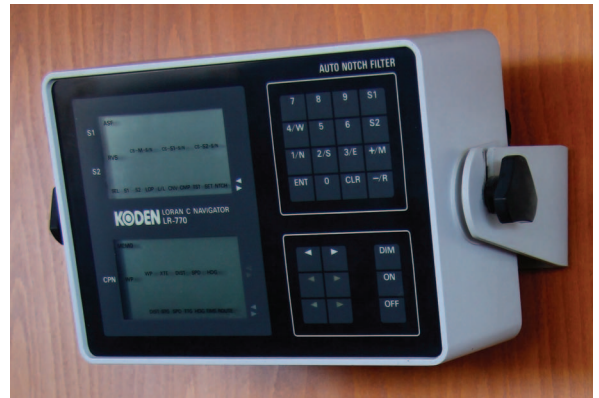
Figure 6. A LORAN-C receiver for use on merchant ships. (Source: Wikimedia Commons: Morn the Gorn.)
