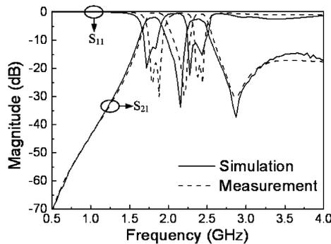
Fig. 6. Simulated and measured results of the proposed DSIR bandpass filter.
