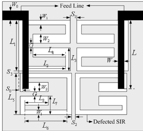
Fig. 5. Configuration of the proposed DSIR dual-band filter. ( $W_0 = 2.8$  mm,  $W_1 = 1.1$  mm,  $W_2 = 1.8$  mm,  $W = 1.0$  mm,  $L = 16$  mm,  $L_1 = 12$  mm,  $L_2 = 7.8$  mm,  $L_3 = 5.8$  mm,  $L_4 = 6$  mm,  $L_5 = 9.1$  mm,  $L_6 = 7.8$  mm,  $L_7 = 4.35$  mm,  $L_8 = 5.5$  mm,  $G = 0.4$  mm,  $S_0 = 0.5$  mm,  $S_1 = 1.2$  mm,  $S_2 = 0.6$  mm).
