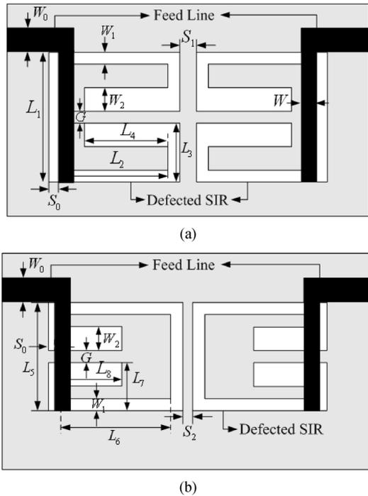
Fig. 3. Configuration of two types of bandpass filter. (a) Filter I. (b) Filter II.
