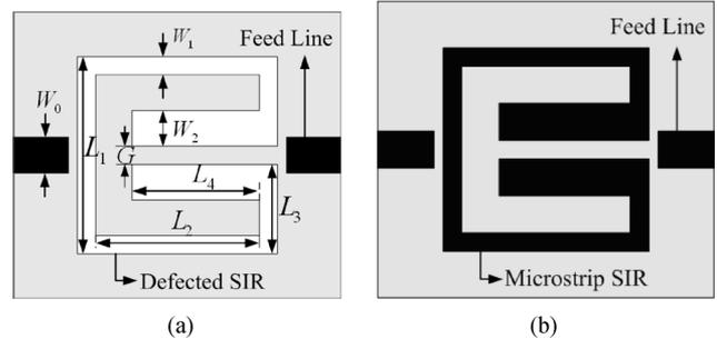
Fig. 1. Structure of microstrip ring resonators. (a) Defected SIR unit. (b) Microstrip SIR unit.
