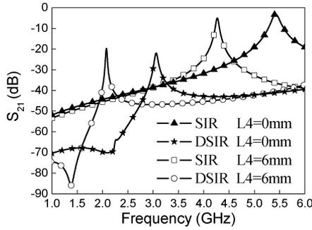
Fig. 2. Resonant property of DSIR and SIR with and without middle loaded stubs. ( $W_0 = 2.8$  mm,  $W_1 = 1.1$  mm,  $W_2 = 1.8$  mm,  $L_1 = 12$  mm,  $L_2 = 7.8$  mm,  $L_3 = 5.8$  mm,  $G = 0.4$  mm).
