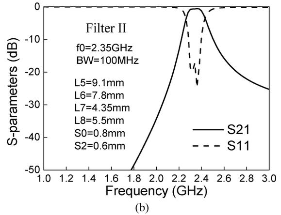
Fig. 4. Simulated results of (a) Filter I and (b) Filter II.
